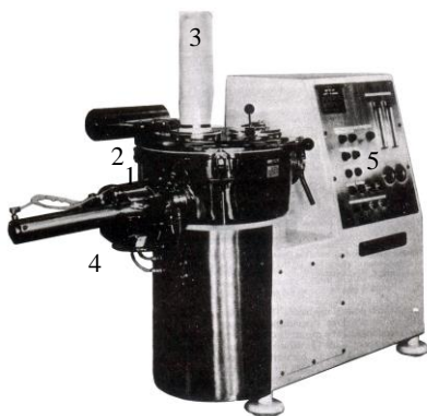
Figure 2.3: Littleford MGT Mixer-Granulator. (1) Bowl; (2) Lid with Counter Weight; (3) Exhaust Sleeve; (4) Discharge Port; (5) Control Panel.
