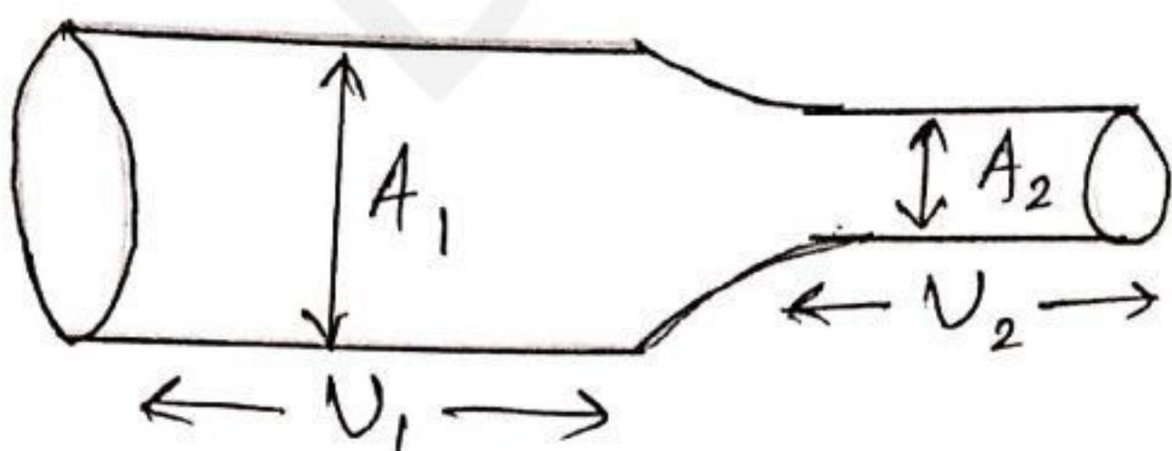
$$\Delta H = \frac{V_2^2 - V_1^2}{2g}$$
