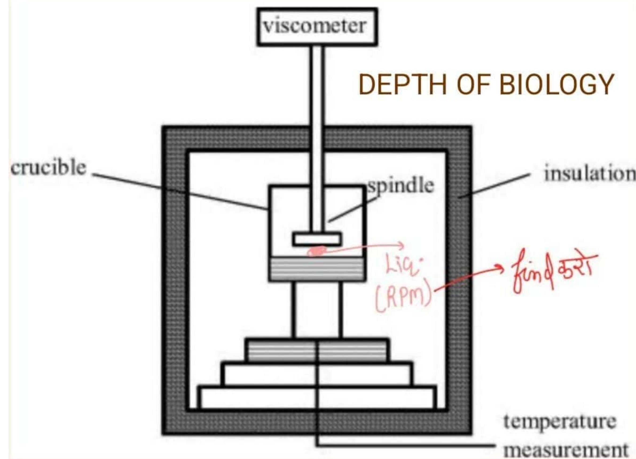
\* This Viscometer are Used for both Newtonian & Non-Newtonian flow.
