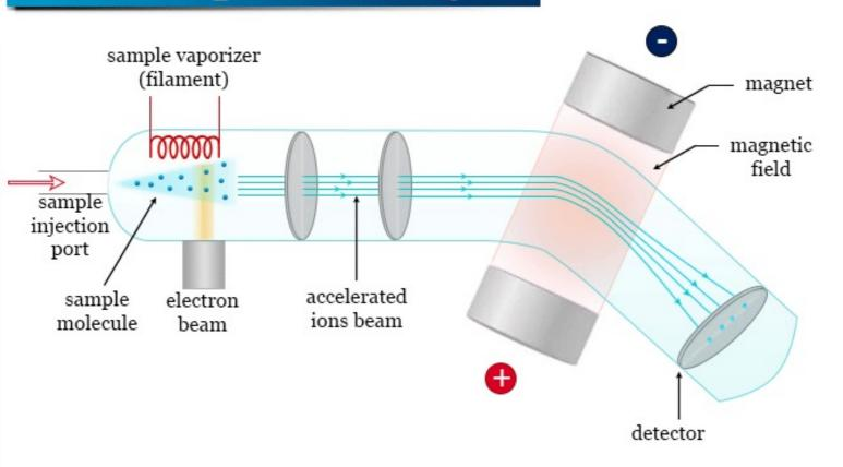
Mass Spectrometry— is a powerful analytical technique used to identify and characterize compounds by measuring their mass—to—charge (m/z) ratios.
