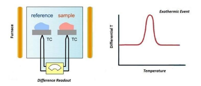
We have two crucibles or sample holders placed side by side in a furnace:
