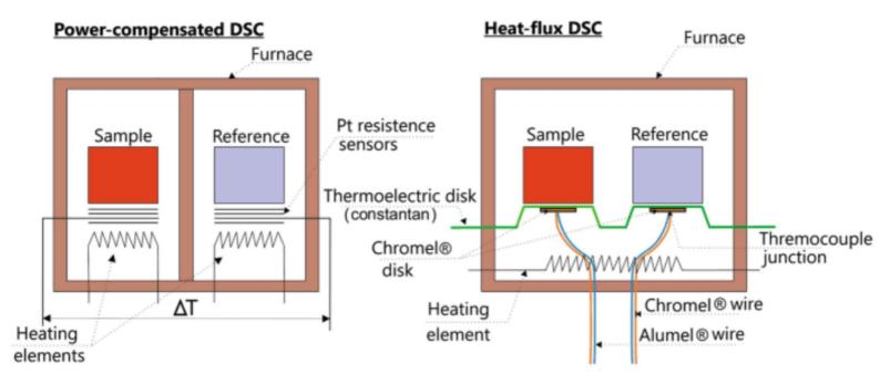
This diagram shows two different types of Differential Scanning Calorimeters (DSC):
